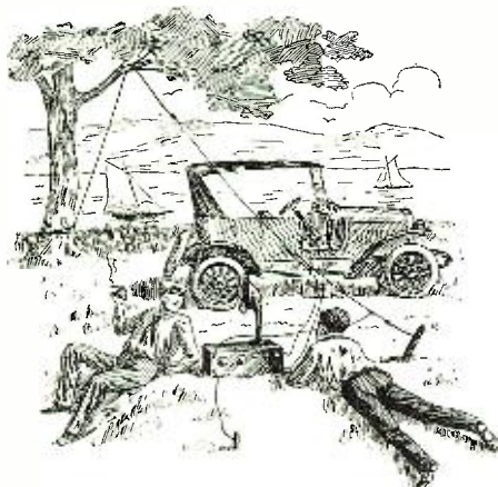
Fig. 5. How the tourist may set up his radio receiving set. The car battery supplies the "A" current for the tubes and a tree supports the single-wire antenna.
