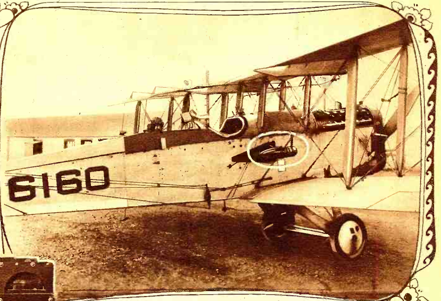
WIND-DRIVEN GENERATOR ON AIRPLANE. In the enclosure is shown the single-bladed and self-regulating generator that supplies power for the radio transmitting and receiving apparatus for Navy airplanes. Courtesy Naval Engineering Dept.
