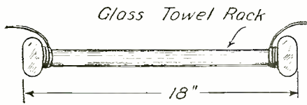
Antenna insulator, which is made from a glass towel-rack.
